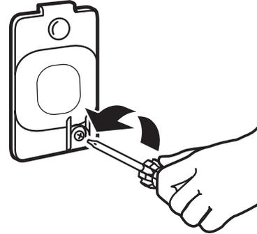
3. Turn bulb counterclockwise. Replace the bulb with a 10 W appliance bulb only. Replace the cover and secure with the screw.
