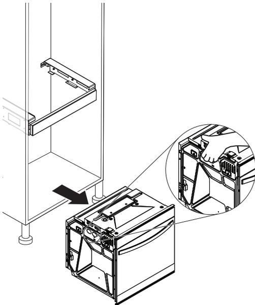
9. Using two or more people, lift the upper oven by the side handles located on the right and left side of the oven. Gently insert into the cabinet cutout, sliding it on top of the left and right brackets.
