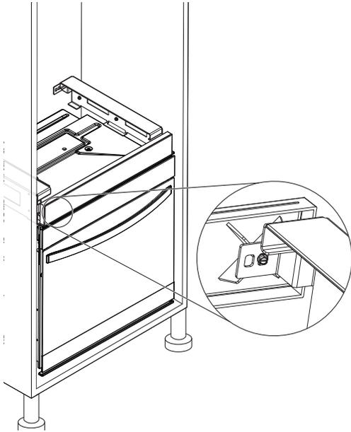
8. Using two or more people, gently remove the lower oven outside the cabinet using the handles located on the right and left side of the oven.
