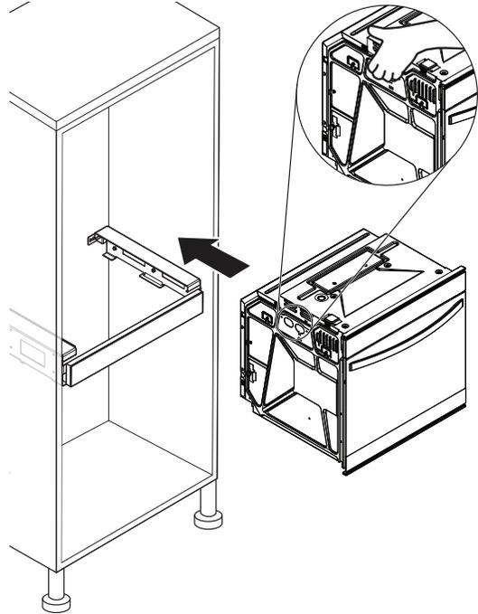
10. Push against seal area of front frame to push oven into cabinet.
