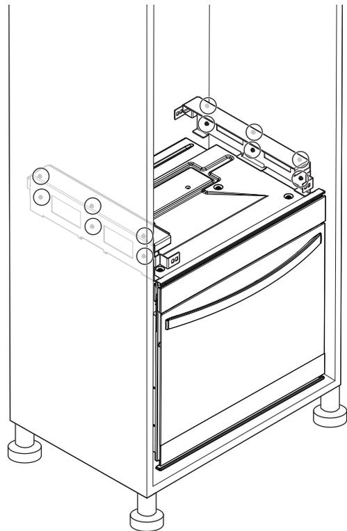
7. Screw the aesthetic panel to the front bracket flange using the remaining two 4 x 12 mm screws.
