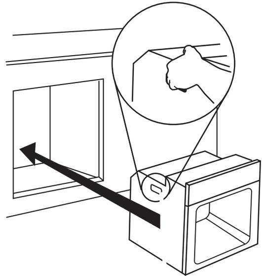
2. Push against seal area of front frame to push oven into cabinet.
