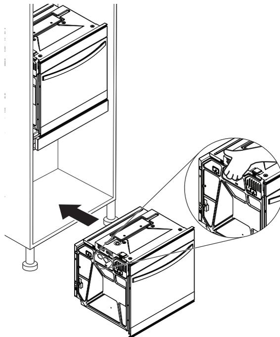
2. Push against seal area of front frame to push oven into cabinet.
