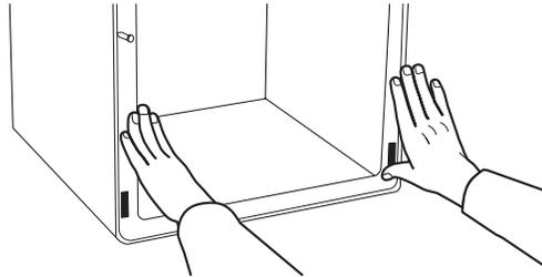
11. Using two or more people, gently move the lower oven by the side handles located on the right and left side of the oven and place on the floor near the cabinet opening.
