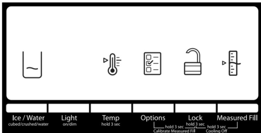
For your convenience, your refrigerator and freezer controls are preset at the factory. When you first install your refrigerator, make sure that the controls are still set to the recommended set points. The factory recommended set points are 37°F (3°C) for the refrigerator and 0°F (-18°C) for the freezer.
