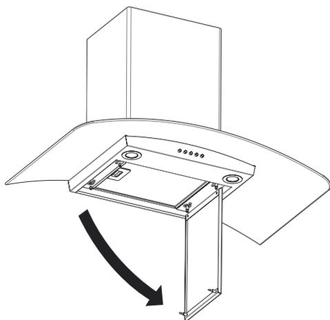
2. Remove the filter by pulling the spring release handle and then pulling down the filter.
