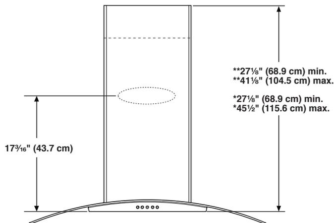
The chimneys can be adjusted for different ceiling heights. See the following chart.
