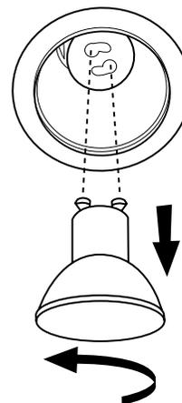
3. Remove the bulb and replace it with a 120 V~, 7.5 W maximum LED bulb with a GU10 base. Turn it clockwise to lock it into place.
