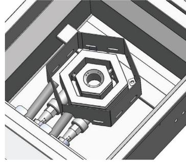
The knob on the left controls the outer burner ring and the knob on the right controls the inner burner ring.
