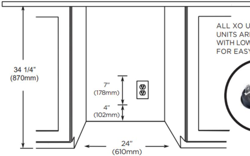
ALL XO UNDERCOUNTER UNITS ARRIVE PRE-WIRED WITH LOW PROFILE PLUGS FOR EASY INSTALLATION
