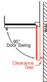
WHEN INSTALLING WITH THE HINGE SIDE NEXT TO A WALL - LEAVE ADEQUATE SPACE FOR CABINET HANDLES
