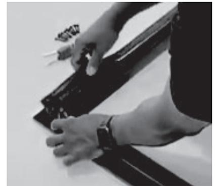
4. Starting at one corner, gently pull the rubber door gasket out of the channel. Lay it aside, flat. You will reinstall it shortly. In the channel are 10 screw holes.
