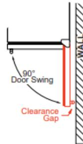
WHEN INSTALLING WITH THE HINGE SIDE NEXT TO A WALL -
